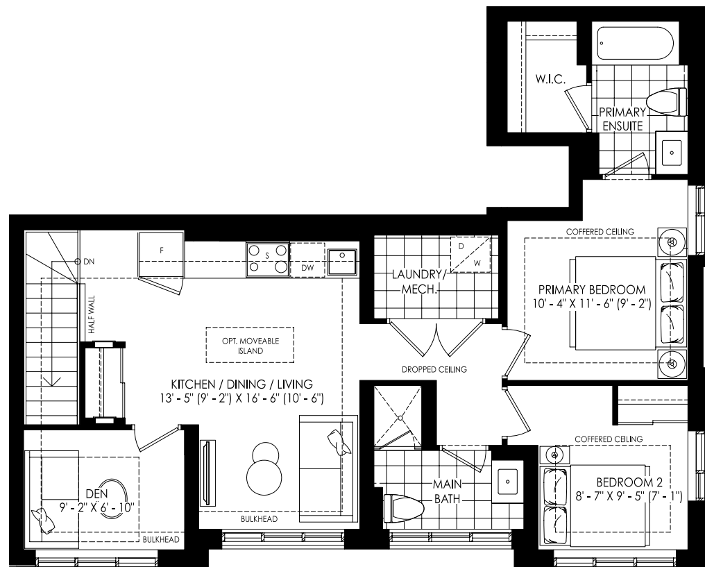
SECOND FLOOR (8 FEET CEILING)
